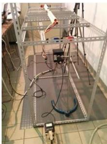
Fig1: Picture of the neutron probe and tennoluminescent detectors around the prototype
